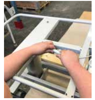
3. Disconnect the actuator cable/cables and remove the stretcher.
