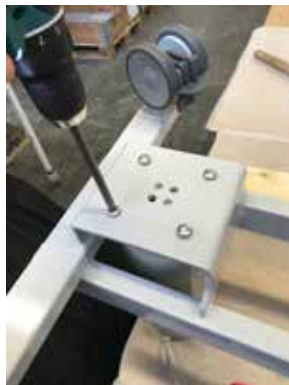
5. Turn the chassis around and remove the four M8x30D bolts that are attached to the column from underneath.
