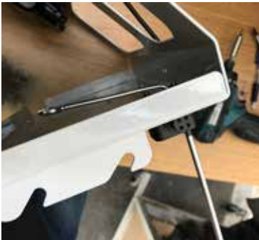
4. Unscrew the bracket holding the control box connector.
