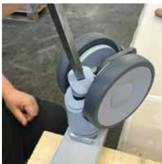
7. Assemble the cap by pressing it and turn it clockwise with a screwdriver.
