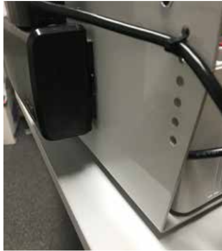
2. Cut the cable ties holding the hand control cable.
