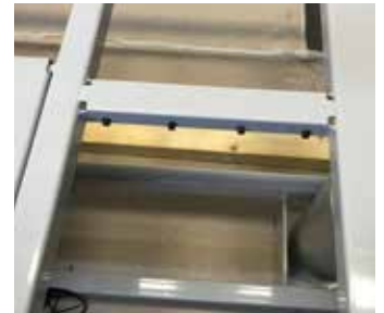
10. Fasten the cables with plastic stripes again and the put plastic plate and mattress back on the stretcher.
