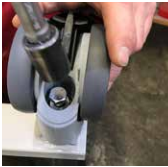
2. Unscrew the bolt and remove the castor.
