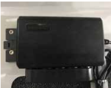
7. Push the new control box to the left to fasten in it onto the plastic bracket. A click sound will be heard when its in position.
