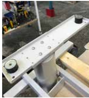
8. Turn the chassis around and fasten the columns with four M8x30 bolts on top.
