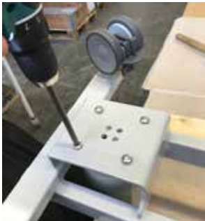
7. Fasten the actuators from underneath with four bolts.
