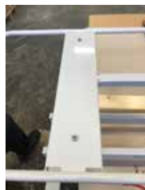
7. Fasten the stretcher with the four M10x12 bolts.
