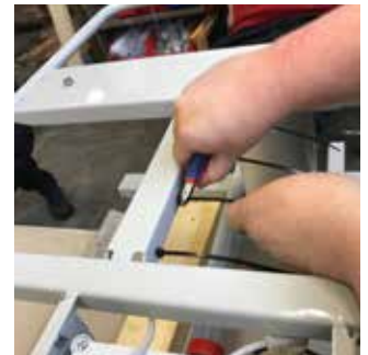
12. Fasten the cables with plastic stripes again and put plastic plate and mattress back on the stretcher.
