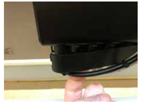
3. Remove the bracket on the control box.
