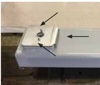
4. Place the straight steering plate onto the chassis. Note the position of the angle on the plate and the pins.
