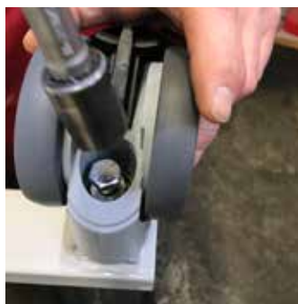
2. Unscrew the bolt and remove the castor.
