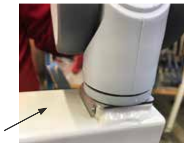
5. Place the castor plate between castor and chassis. Note the position of the angle on the plate.
