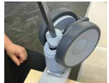
10. Assemble the cap by pressing it and turn it clockwise with a screwdriver.
