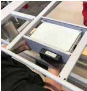
8. Fasten the plate and battery box with the four M5x12D screws.
