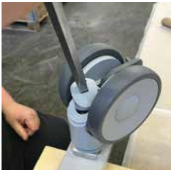
1. Remove the protective cap by turning it counter clock-wise with a screwdriver.
