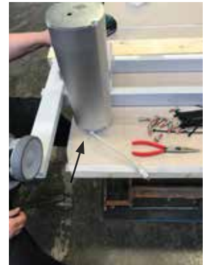
6. Place the lifting column upside down. Note the position of the cables
