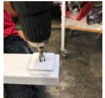
3. If necessary, carefully clean the threads from Loctite with an M10 tap.
