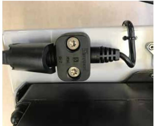
4. Connect the battery to the control box connector.
