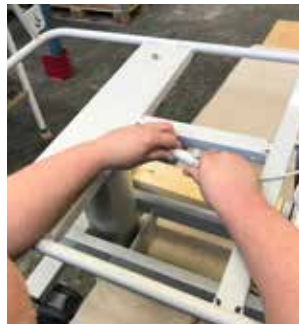
11. Connect the actuator cable with the cable from the control box.
