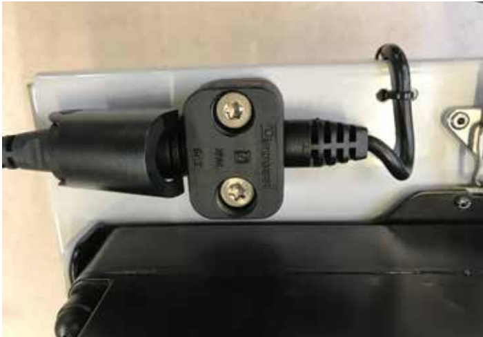
1. Disconnect the battery from the control box connector.
