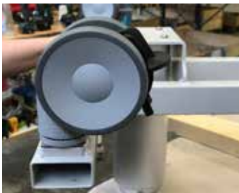
8. The black lever on the straight steering castors shall point inwards (both left and right castor) when the castor is fastened. This will be the position when the straight steering mechanism engages in use.
