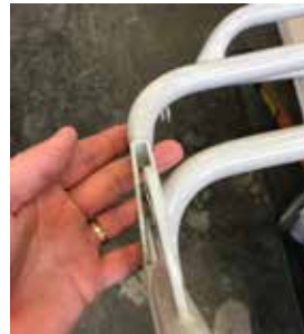
2. Put the side rail ends over the support plate on the stretcher.
