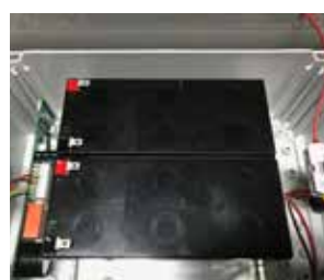
5. Insert the new batteries in the plastic enclosure.
