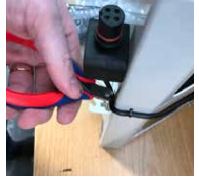
3. Cut the cable ties holding the control box cable.
