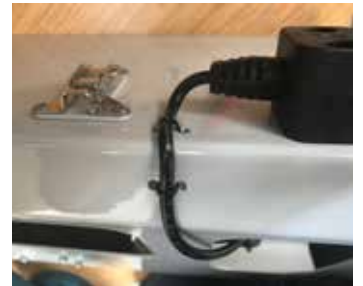
9. Fix the cables with cable ties and attach the hand control- and lifting column connectors.
