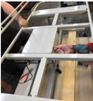
1. Unscrew the four M5x12D screws to remove the metal lid on the stretcher.
