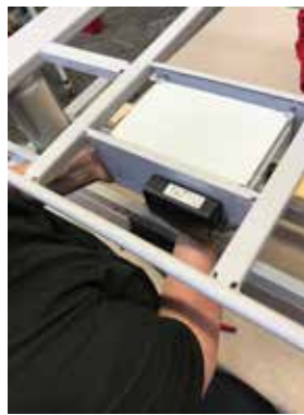
5. Unscrew the plate holding the battery box.
