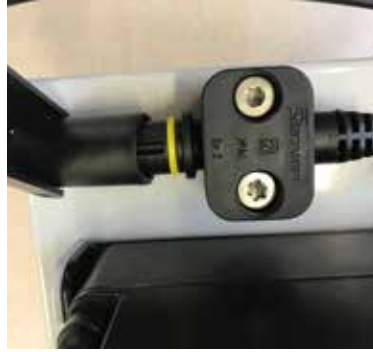
2. Disconnect the battery from the control box connector.
