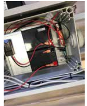
3. Disconnect + and - leads from the circuit board to the battery and also + and - leads from the fuse holder.
