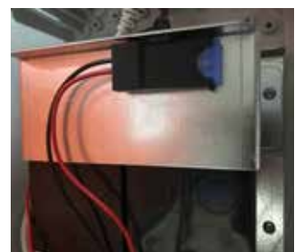
6. Place the bracket on the batteries and fasten it.
