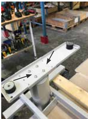
4. Remove the four M8x30 bolts attached to the lifting column and remove the bracket with the dampers.
