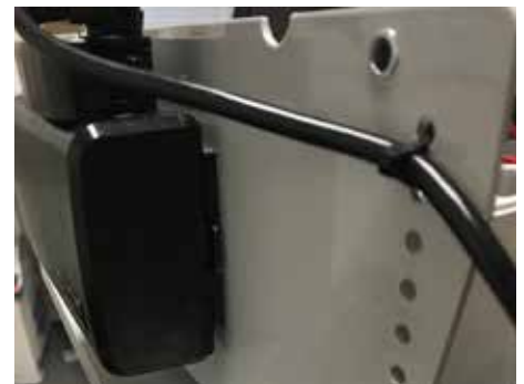
6. Fasten the hand control cable with a cable tie.
