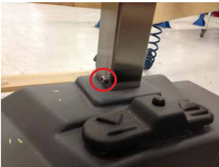
Remove the bolt on the column (Allen Key 5 mm) (TR 9650)
