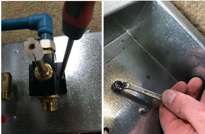
Unscrew the valve bracket by using a Screwdriver and a Spanner.
