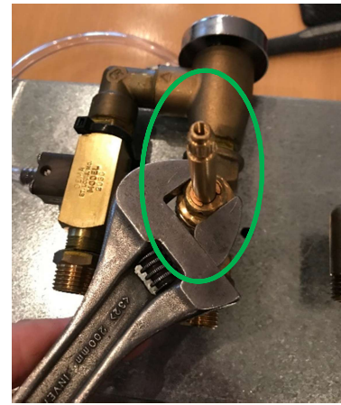
Loosen and remove the Valve stem by using a spanner.
