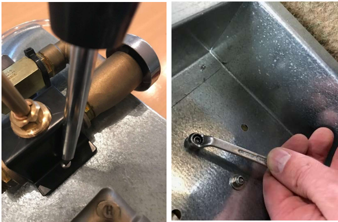
Unscrew the Valve bracket by using a Screwdriver and a Spanner.
